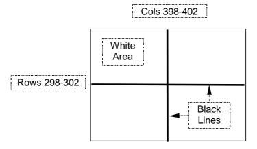
TEST PATTERN FOR IMAGE STICKING TEST
